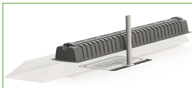
Figure 3.8.2 | Position of the sampling device underneath the sand layer
