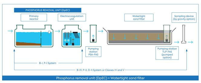
The phosphorus removal unit (DpEC) is composed of a primary reactor and an EC unit.
